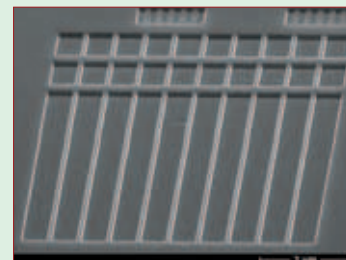
Test structure in mr-I 7000, 200 nm lines
