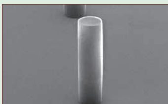
UV imaging of a 300 µm thick SU-8 layer
