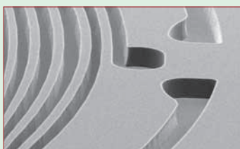
UV imaging of a 30 µm thick micro coil
