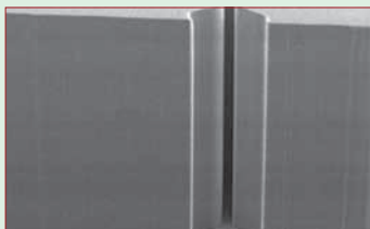
Preparation of a 1000 µm thick resist layer
