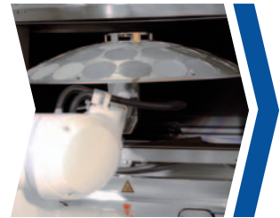
4. Dome transfer through dedicated side port either direct to coater or via loadlock chamber.
